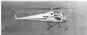
BRANTLY B-2 helicopter has top speed of 150 mph., useful load of 420 lb., and is powered by 180 hp. Lycoming VO-503 A1A.
